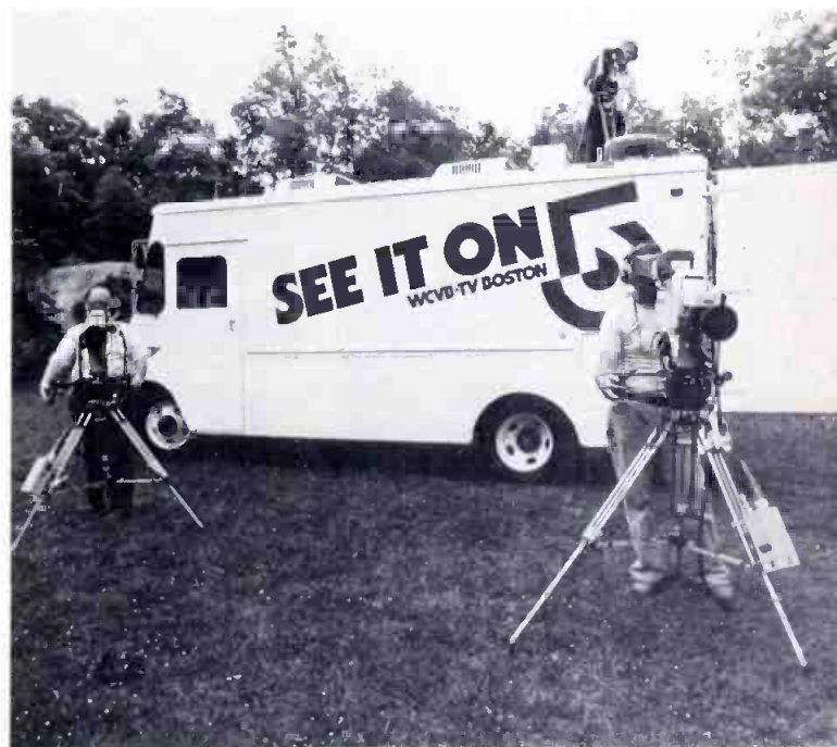
WCBV-TV engineers are pictured manning the three cameras of "The Hippo," a new, compact remote production unit. The roof-mounted RCA TK-76 joins two Ikegami HL-51s for unique production capabilities in a small, maneuverable vehicle.
